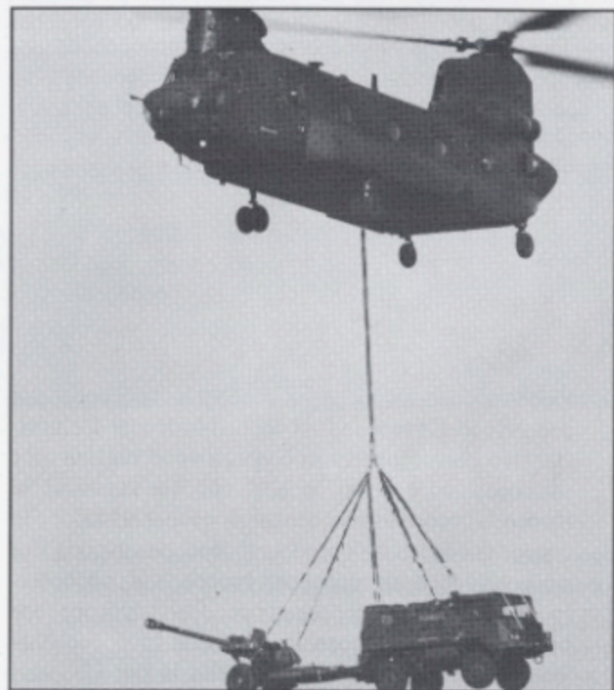
A Steyr and gun of the Regiment underslung beneath a Chinook helicopter in their airmobile role
